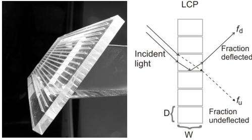
Figure 1: Laser cut panel (left) and Light deflection through a mirror light pipe (right)
