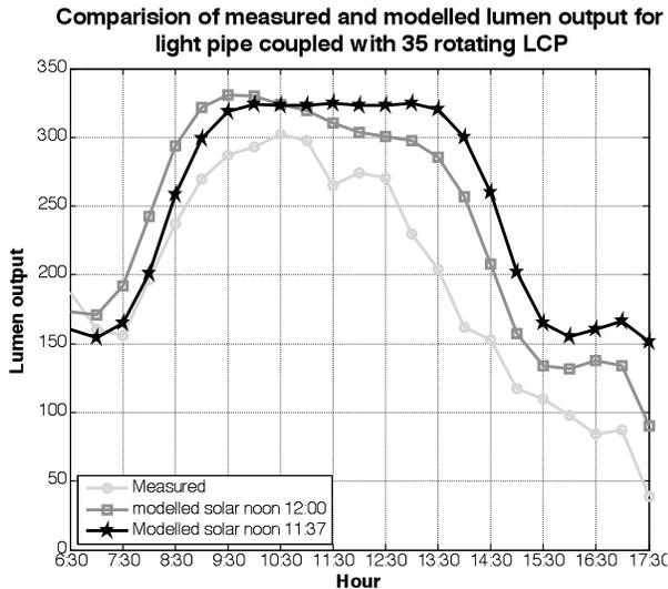
Figure 8: Comparison of measured and calculated lumens out for 24hrs rotating LCP
