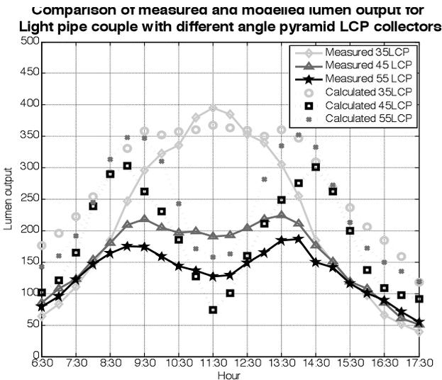
Figure 9: Comparison of measured and calculated lumens out for pyramid LCP at 35°, 45° and 55° tilt.
