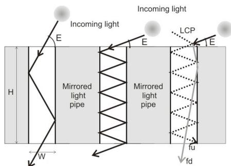
Figure 3: Light transmission through MLP pipe for high elevation angles, and low elevations with and without LCP
