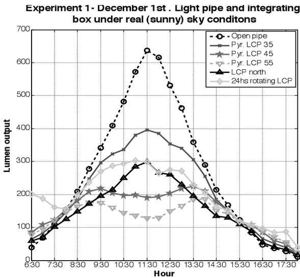
Figure 6: Testing on December 1st, for tracking and rotating LCP collectors, and pyramid LCPs at different tilts.
