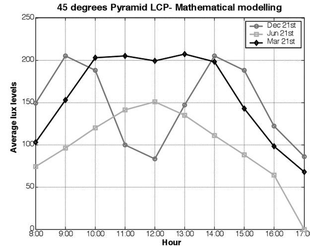
Figure 11: Modelling of pyramid LCPs at a 45° tilt for December 21<sup>st</sup>, June 21<sup>st</sup> and March 21<sup>st</sup>
