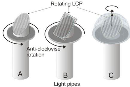
Figure 4: Rotating LCP collector
